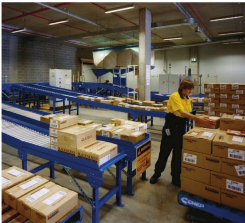
Once past the check-weighing system, cases for completed orders are conveyed to a sorter and automatically diverted down one of four shipping lanes for palletization and shipping.
