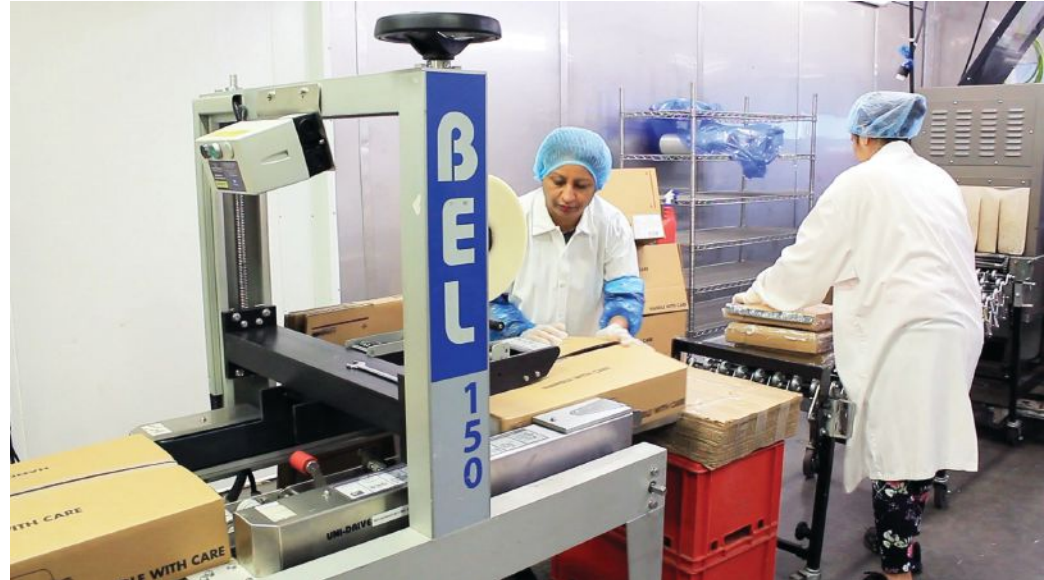
The semi-automatic Bel 150 case taper from Wexxar Bel can seal a wide range of case sizes at speeds up to 30 cases per minute, while facilitating quick case size changes.
