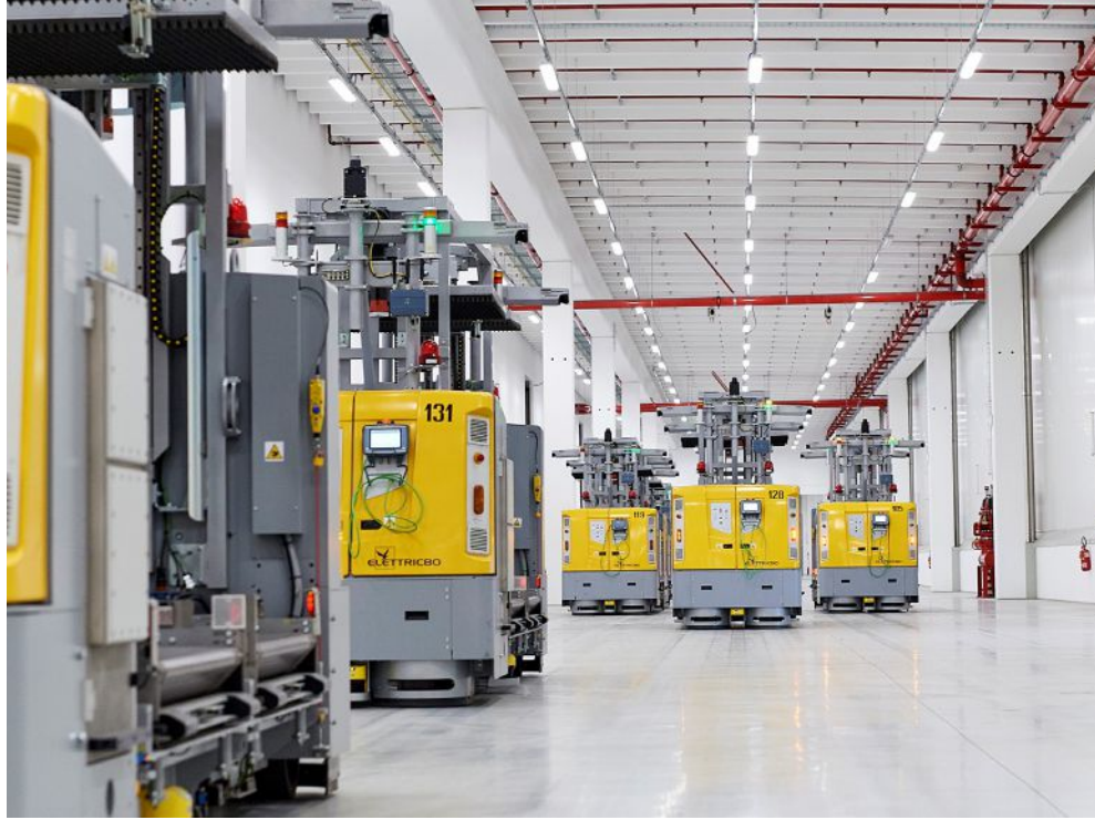
Barilla's Parma pasta factory and distribution facility currently employs a fleet of 120 laser-guided vehicles for all of its product transfer needs, essentially eliminating the need for traditional conveyors.
