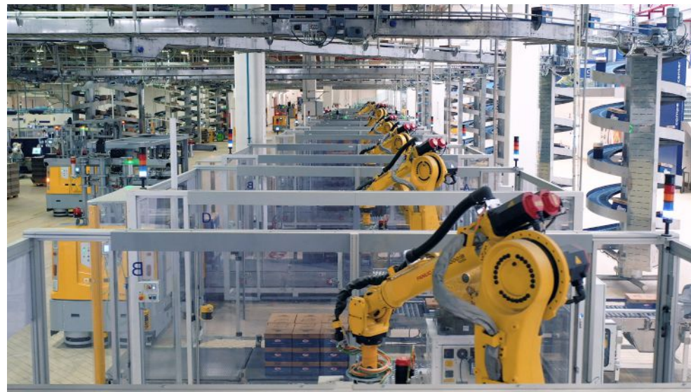
A long row of robotic palletizing workcells perform the unique pallet-less load stacking and layering around-the-clock without the use of any traditional wooded pallets.
