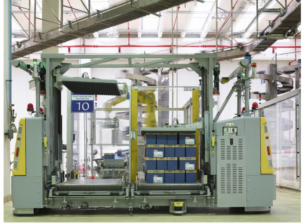
Supplied by automation experts E80, the LGVs used at the Parma plant incorporate innovative rooler-bed design to ensure efficient and safe roll-on/roll-off procedures.
