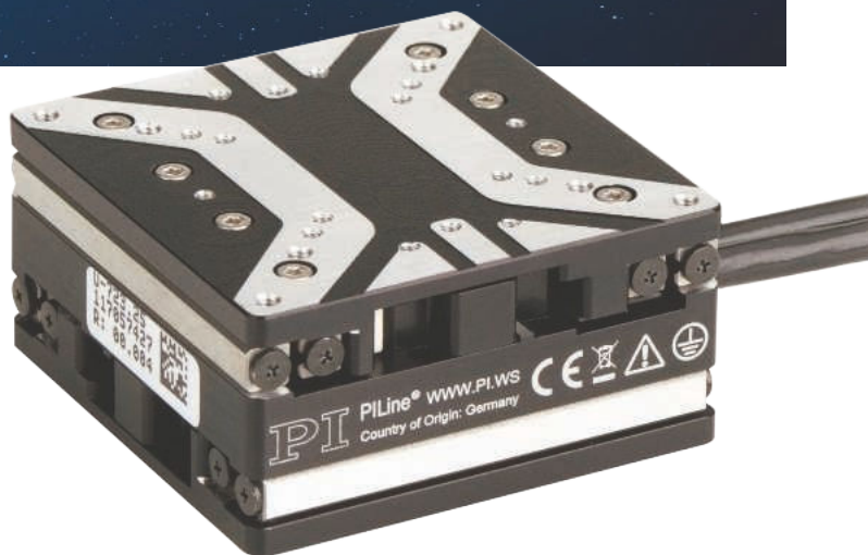
► A miniaturised integrated X, Y stage, which is driven by closed-loop ultrasonic ceramic linear motors and provides high-speed motion with 20 nm resolution over a travel range of 22 x 22 mm. ► Image courtesy of Physik Instrumente (PI).
