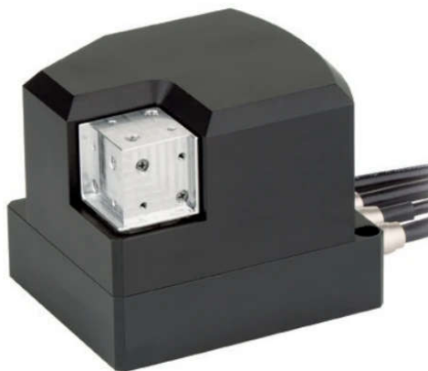
■ Figure 2a (above): NanoCube 6-Axis Nanopositioning and scanning stage based on piezo flexure drives. Piezo flexure stages are available with up to 6 degrees of freedom, allowing fast and highly precise scanning, positioning and alignment with virtually unlimited lifetime due to the non-wear and zero-friction design. (Image courtesy PI). ■ Figure 2b (right): Application of compact XYZ piezo flexure scanning stage in the TERA-print® E series, mask-free, high resolution desk-top nanofabrication tool, a 2020 Prism Award winner. (Image courtesy TERA-print).
