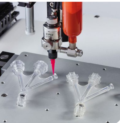
FIGURE 8: xQR4IV needle valve dispensing UV-cure material onto a medical device. Image courtesy Nordson EFD
