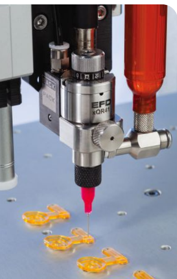
FIGURE 1: Contact dispensing with the xQR41 Microdot needle valve applying UV-cure material onto diagnostic test strips
