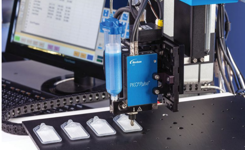
FIGURE 7: Pico Pulse jet valve dispensing medical fluid onto dialysis filters with a 37 ga Microdot dispenser. Image courtesy Nordson EFD
