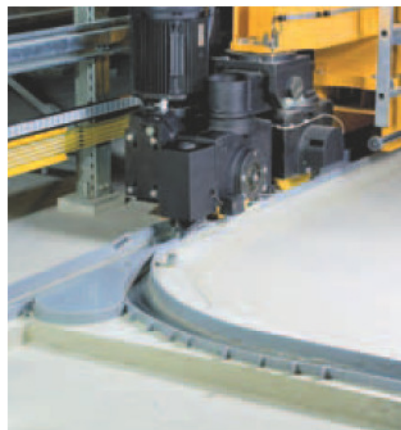
A curved track allows stacker cranes in Catalent's facility to change aisles easily.
