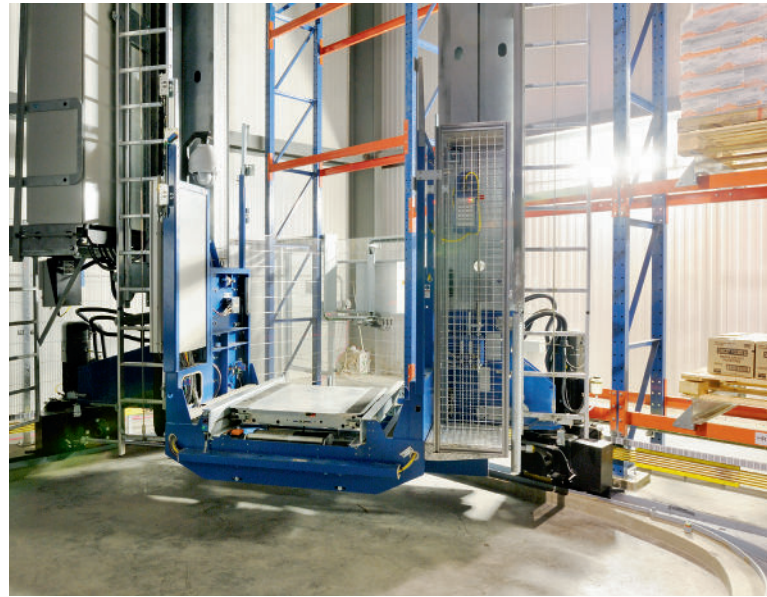
The crane smoothly rotates around the end of the aisle on a curved track.
