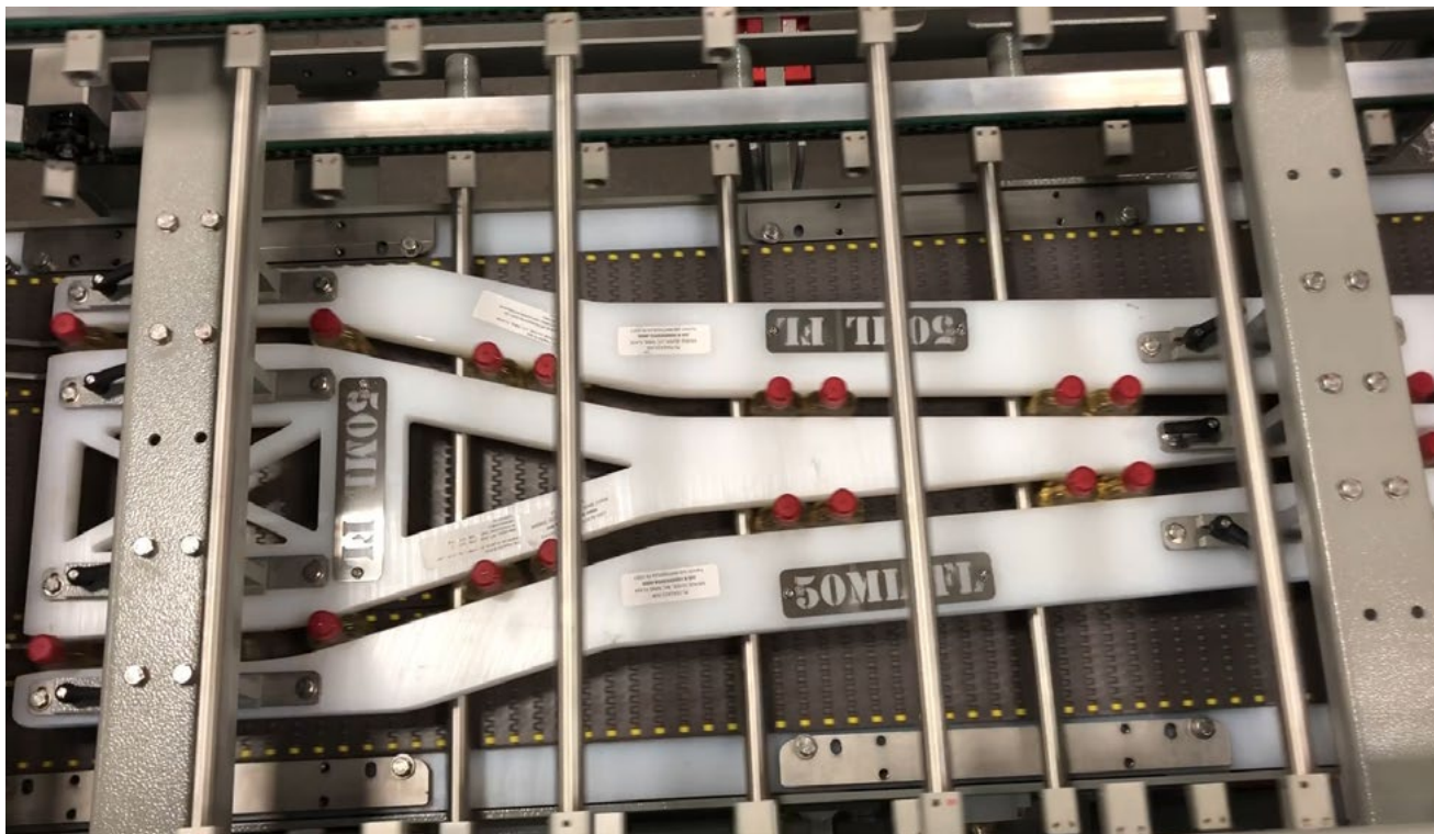
The jaws of the 914 OVS orbital shrinkwrapping system from Texwrap can accept bottles of up to nine inches in height.
