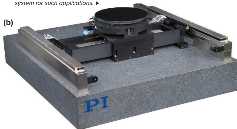
► Figure 3: (a) A comparison of air bearings and mechanical bearings. (b) Wafer dicing requires high accuracy. The permissible tolerances along the travel range amount to only a few micrometres per metre. A planar air bearing stage, which is driven by linear motors, is a suitable positioning system for such applications. ►
