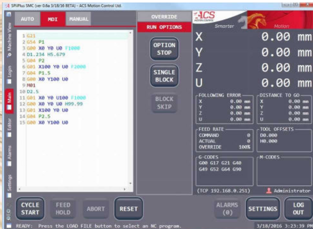
► Figure 9: The human machine interface (HMI) is an important subsystem of the machine and normally falls into one of two classifications. First, and as shown above, there is the CNC style HMI that imports and executes machine-coded programs (typically G code) created by a CAM software post processor. Second, and as shown below, there is the integrated graphical interface. Some HMIs allow importing as well as processing of CAD files and offer integrated functionality for post-processing of the CAM data. (Images courtesy of ACS Motion Control). ►
