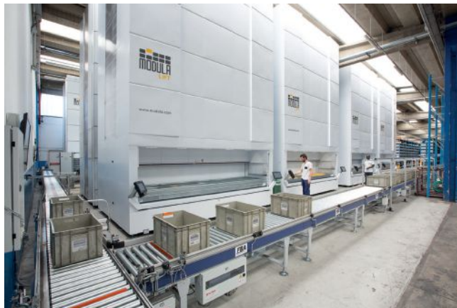
Vertical lift modules providing automated fulfillment for e-commerce orders.
