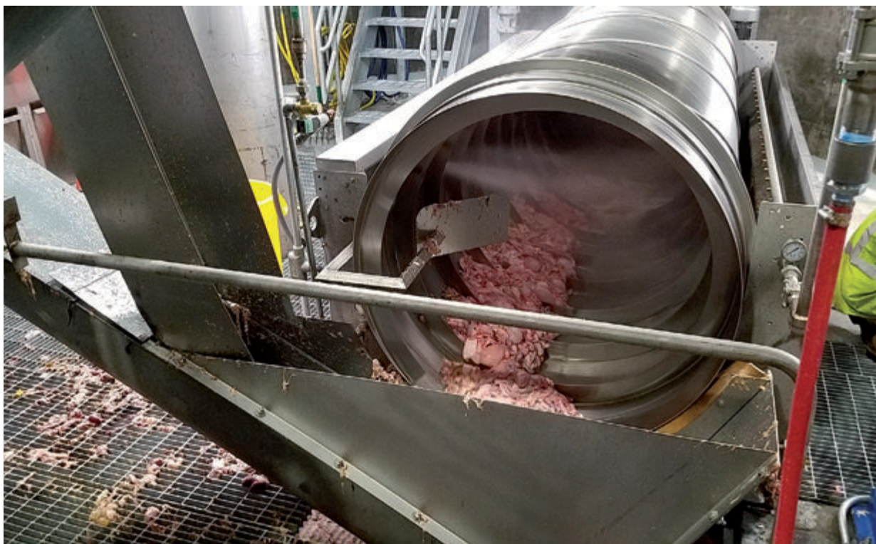
The single-rotary-drum Lyco screens at the Virginia Poultry are very robust, and are very well constructed.
