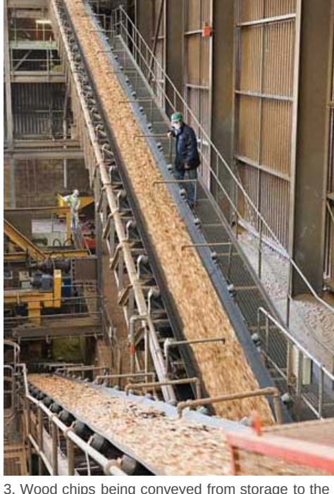
3. Wood chips being conveyed from storage to the plant's two circulating fluidized bed
