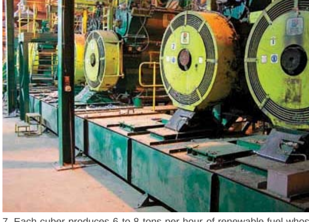
7. Each cuber produces 6 to 8 tons per hour of renewable fuel whose heating value is two-thirds that of the average coal. Courtesy: Slough Heat & Power
