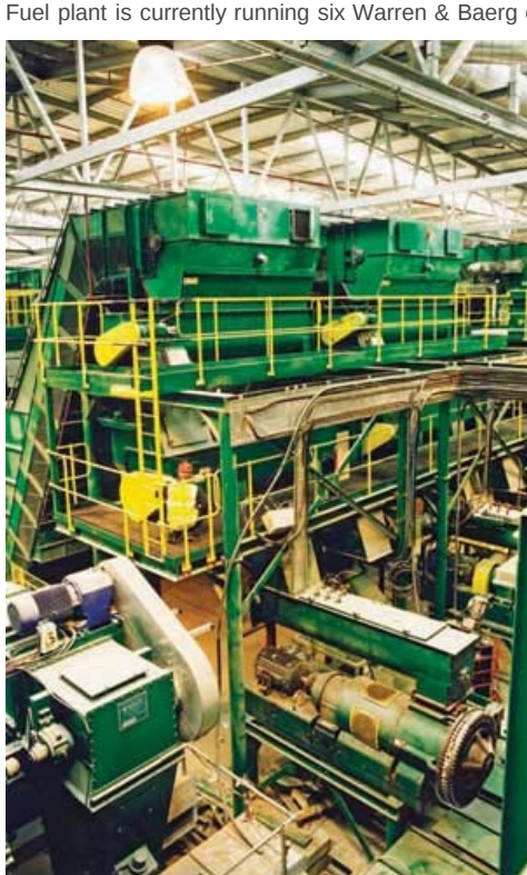
6. The fuel "cubers" supplied by Warren & Baerg produce cubes that are 1.25 to 2.5 inches wide and 3 inches long. Courtesy: Slough Heat & Power
