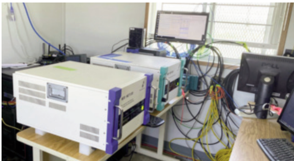
Fiber optic interrogator units that are connected to fibers that run down the wellbore for thousands of feet. Image courtesy Neubrex Ltd
