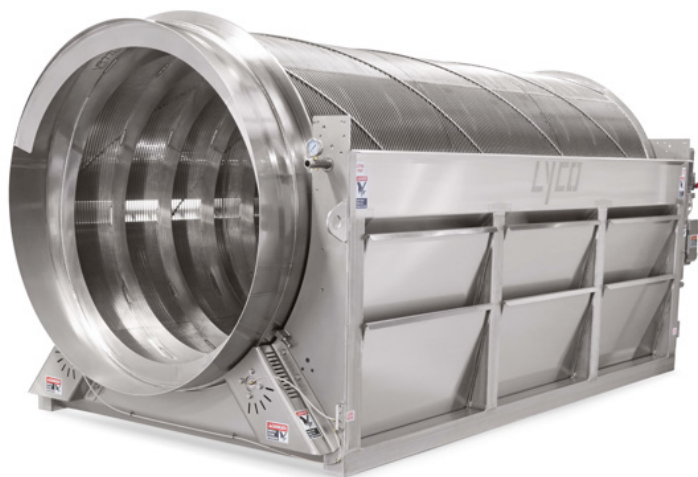
The screens utilize rotary action to separate turkey solids from the water
