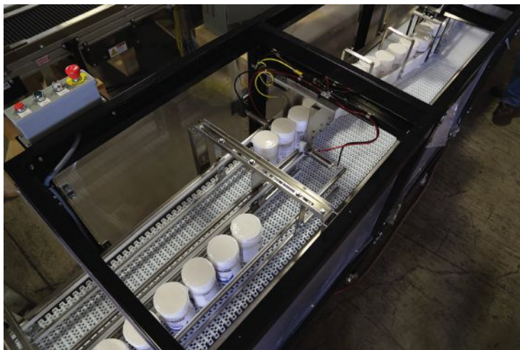
Figure 4: Wet wipes can be moved from one conveyor traffic lane to another traveling in the same or the opposite direction. Courtesy: Shuttleworth
