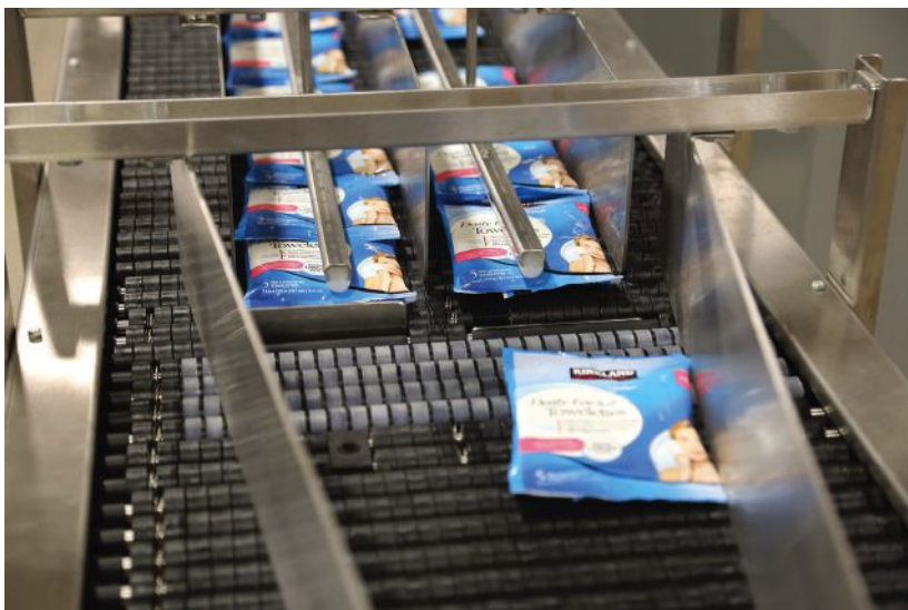
Figure 3: Wet Wipes can be moving at variable speeds on different sections of the conveyor as dictated by throughput requirements. Courtesy: Shuttleworth
