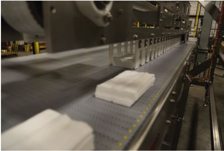
Figure 2: High-speed automation for wet wipes folding, wetting, cutting and piling presents throughput challenges. Courtesy: Shuttleworth
