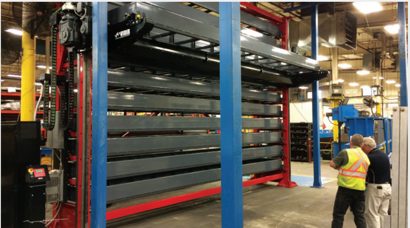
The machine can be adapted for the storage of bar stock, press brake dies and punches
