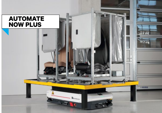
Low-profile AMRs can tunnel easily under tables, carts, racks and shelves.
