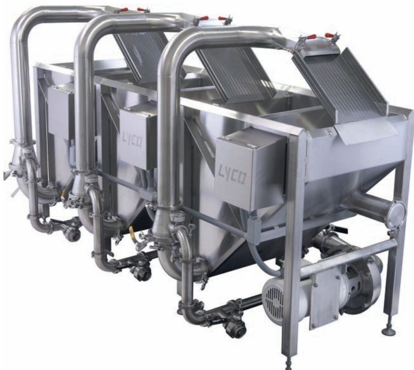
Multi-stage quench systems can reduce product temperature from 200 to 60°F (93 to 15°C) in 21 sec.
