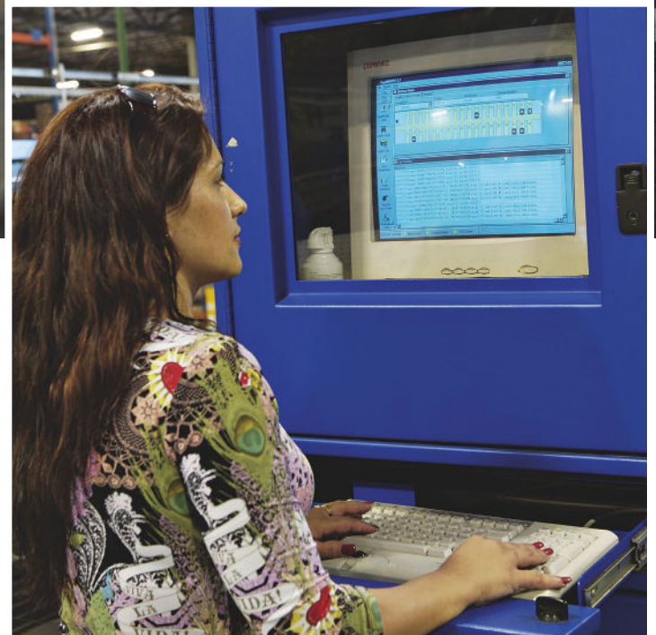
The hub of the Robbinsville distribution center, and where the DC realizes its most profound efficiencies, is with its sortation and conveying systems, which reduce manual labor, top. The SortDirector® warehouse control system, above, integrates with the Robbinsville WMS and coordinates all product movement inside the DC.
