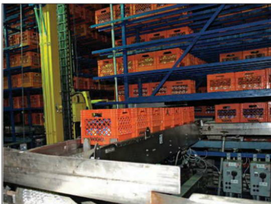
Wawa's mini-load stacker cranes move crates in and out of the 80,000-location high-bay.
