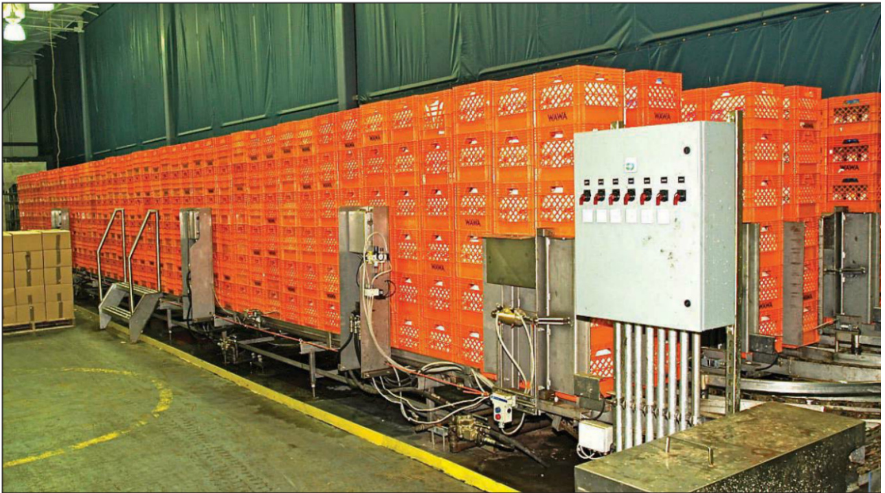
Wawa's distribution facility can automatically handle 42,000 crates of liquid products daily.
