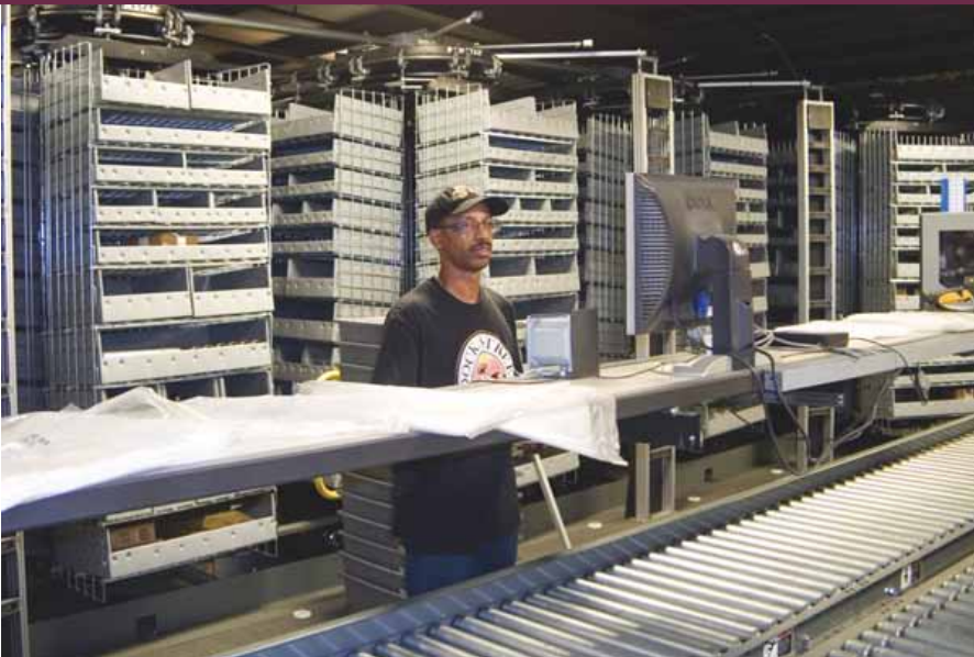
The carousel system consists of 10 carousels and manages an inventory of 60,000 SKUs.
