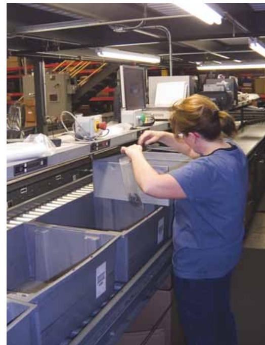
Totes are automatically delivered to operators, who are directed by pick- and put-to-light technologies.
