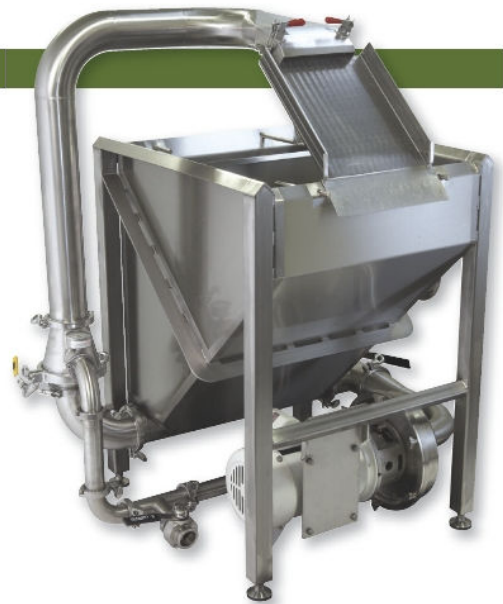
The Easy-Flow quench cycle uses unheated ambient temperature tap water to capture much of a product's heat before it enters the primary chill cycle.
