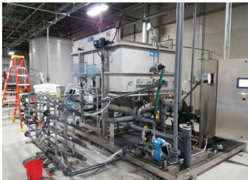
FRC designed Plochman's DAF system to fit into the facility's tight space constraints.
