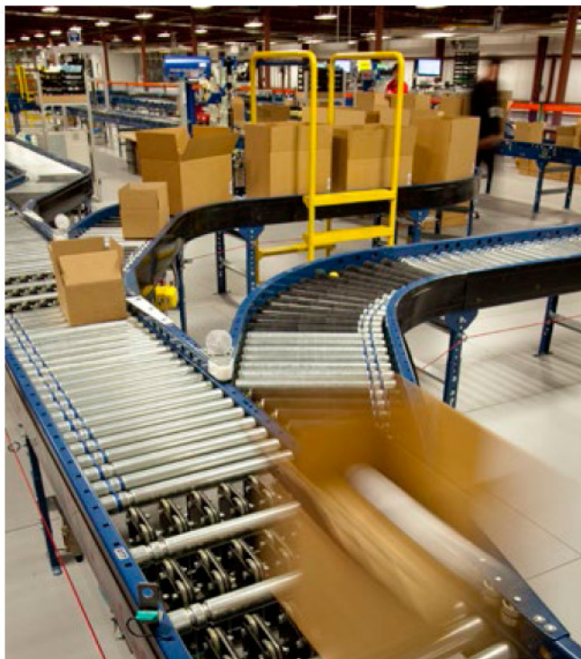
Automated and synchronized pack-out processes in Nature’s Way’s McCarran distribution center enable a single pack line to process 5,000 cartons during an eight-hour shift.
