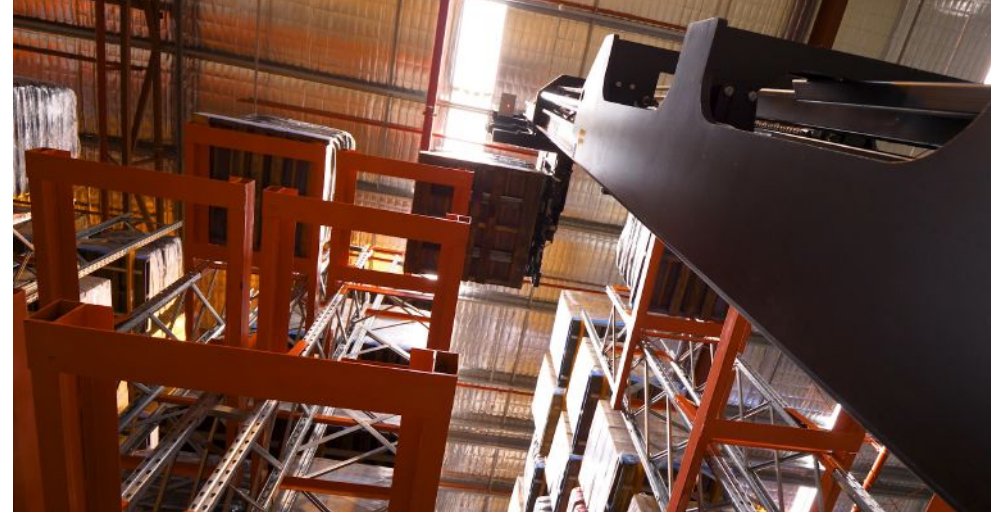
The Elettric80 LGVs can accommodate both single- and double-deep racking, as well as extended depths, with satellite remote units.
