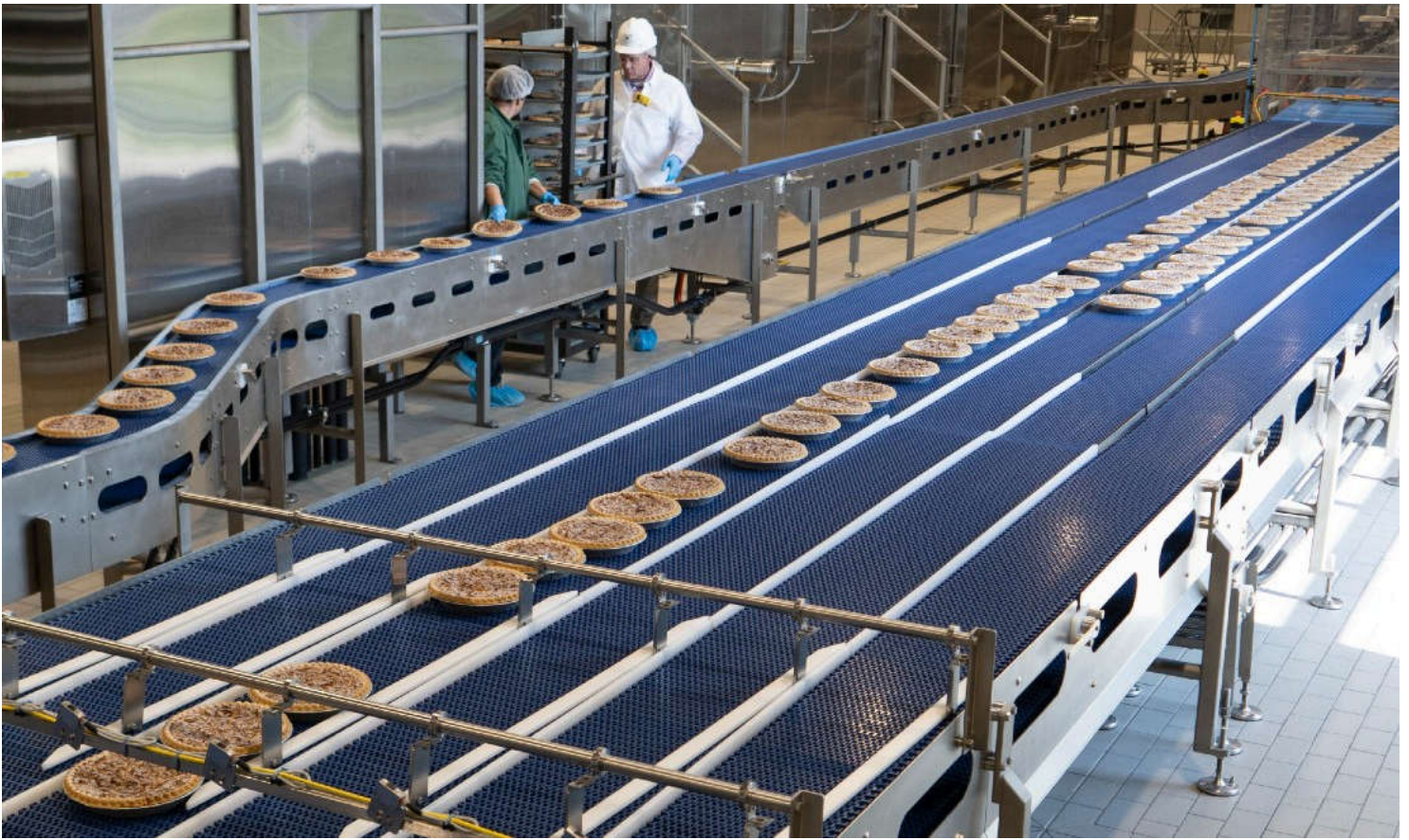
Accumulation of pies after freezing. Image courtesy Gardner Pie
