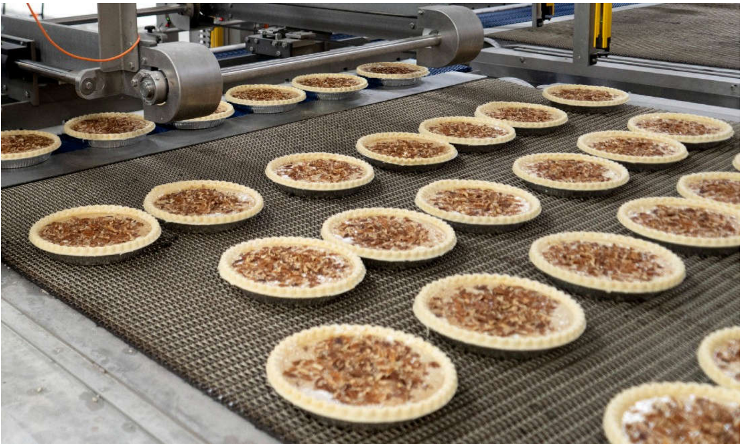
Automated infeed of pies into the oven. Image courtesy of Gardner Pie Company
