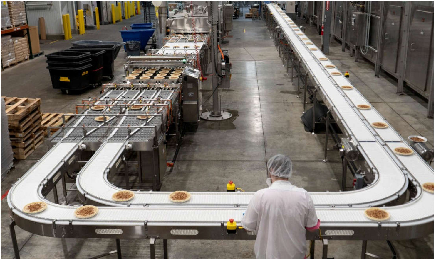
Gardner Pie's conveyor flow from filling to oven. Image courtesy of Gardner Pie Company
