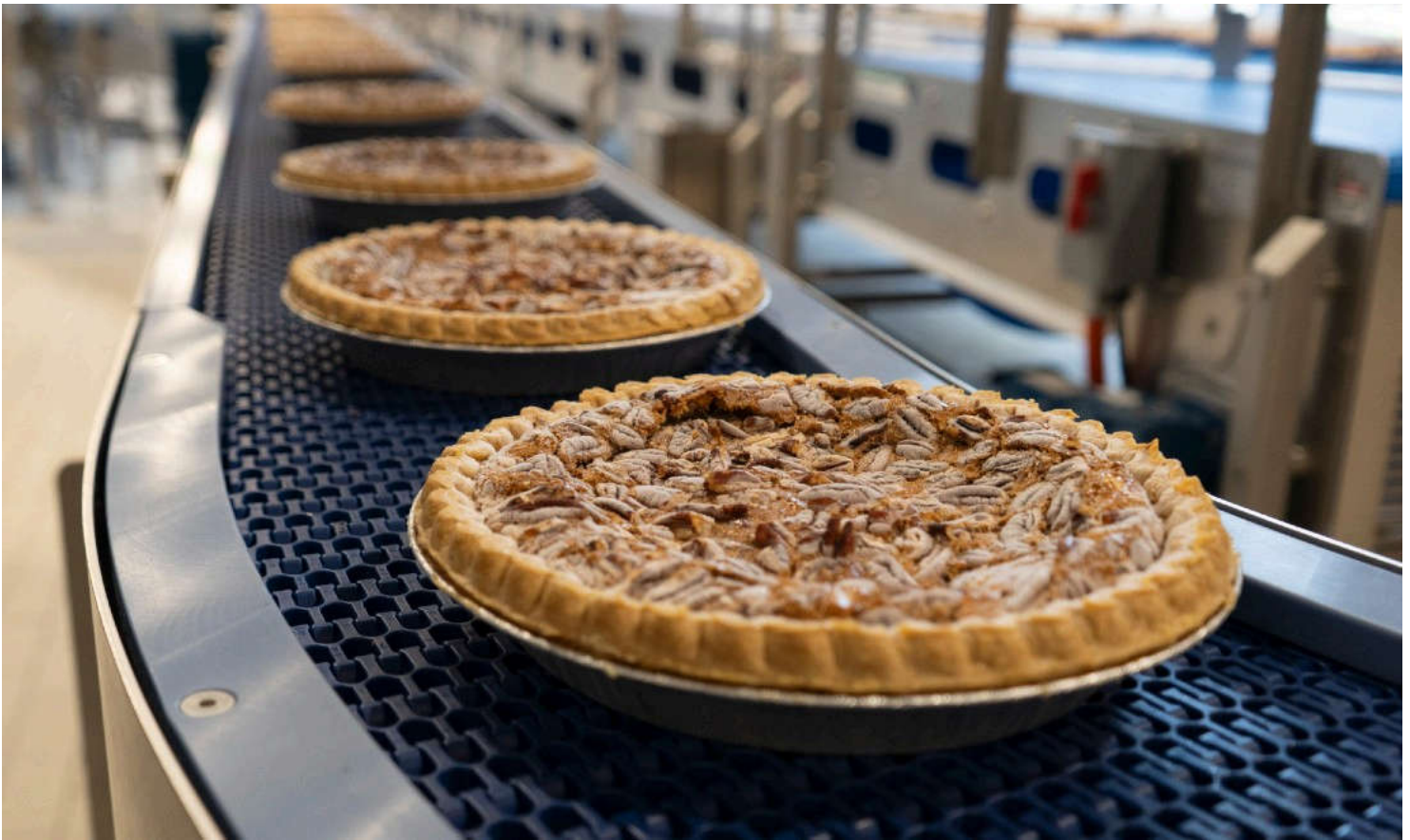
After accumulation, pies are singulated for primary packaging. Image courtesy Gardner Pie
