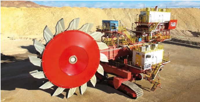
Bucket wheel excavator SR800P9, leached copper ore 9650 m³/h, 14500 t/h, Chile
