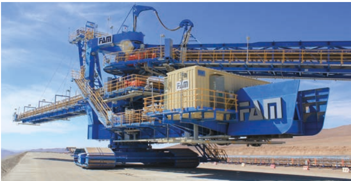
Spreader ST3500.40, compact-type, leached copper ore 3500 t/h, 1950 m³/h, Chile
