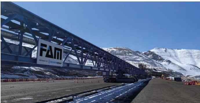
Conveyor bridge on crawlers MSB1000.9, leached gold ore 1000 t/h, Chile
