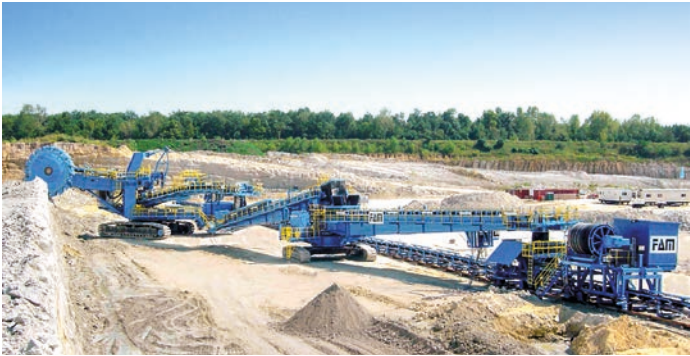
Transfer conveyor on crawlers BW1200.22/28R, bridging length 50 m, marl 2300 t/h, 1600 m³/h, USA
