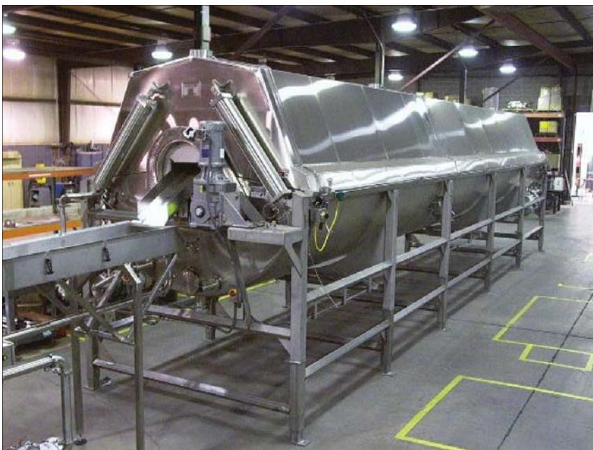
Fig. 1. The Hydro-Flow applies a combination of air and water injection which physically and buoyantly supports heavier loads.
