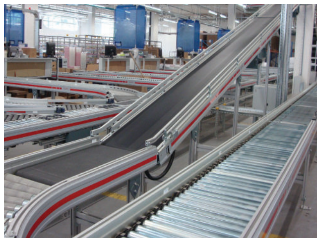
Conveyor system for cartons and totes
