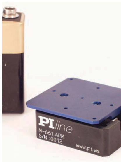
Miniature translation stage with ultrasonic linear motor compared to a 9V block battery. This unit provides 0.8 inch of travel with speed to 20 inch/sec, and 10g acceleration. A high-resolution linear encoder is also integrated. Smaller versions are feasible.
