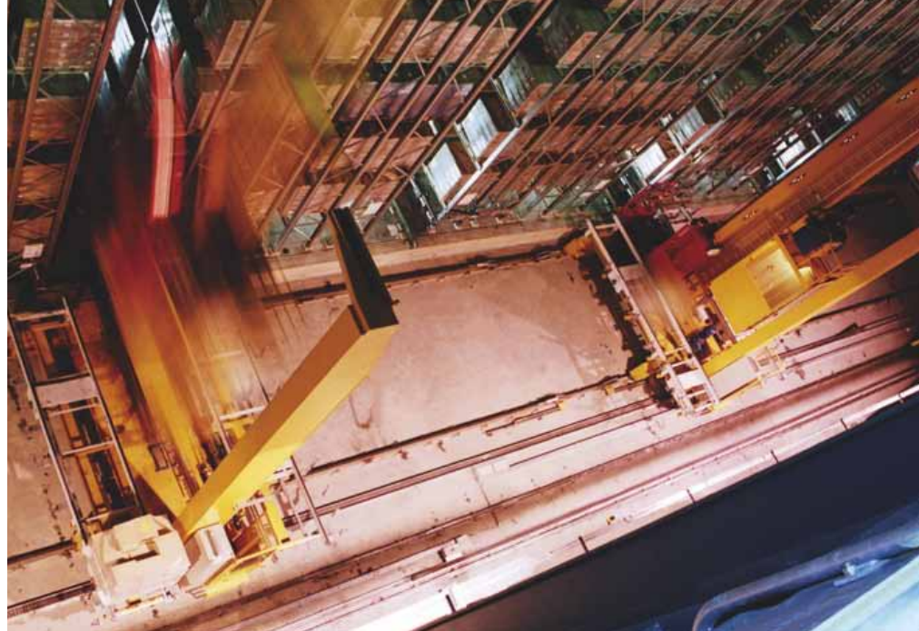
Two of the 17 storage-and-retrieval cranes in the finished-goods store, which has more than 12,000 pallet-storage locations.
