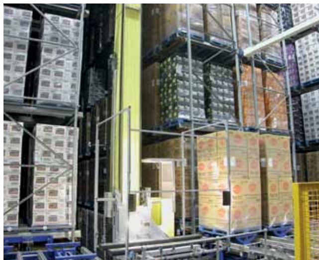
Double-deep storage of packaged food manufacturer
