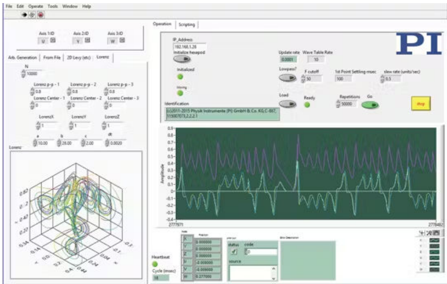
Figure 4: A complex motion profile is programmed using a multi-axis patterned motion tool, as demonstrated in this graphic user interface (GUI) environment. (Courtesy of PI)
