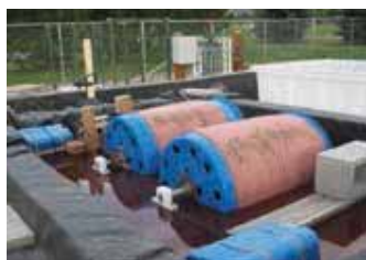
Left: Outdoor RABRs in produced water for cultivating and harvesting microalgae, at inoculation. Right: Outdoor RABRs in produced water for cultivating and harvesting microalgae, 21 days later. Photos by WesTech Engineering
