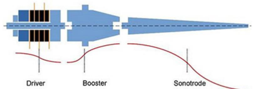
ratio of the cross-sectional areas at both ends of the sonotrode. In medical technology, working frequencies of 20kHz to 100kHz are used and the geometry of the entire scaler is designed accordingly in multiples of half of the wavelength.
