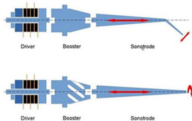
Figure 4: Scaler with angled sonotrode and spiral sonotrode.
