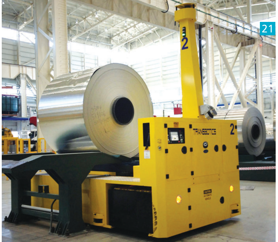
60,000 pound aluminium coil being loaded onto a lightweight AGV
