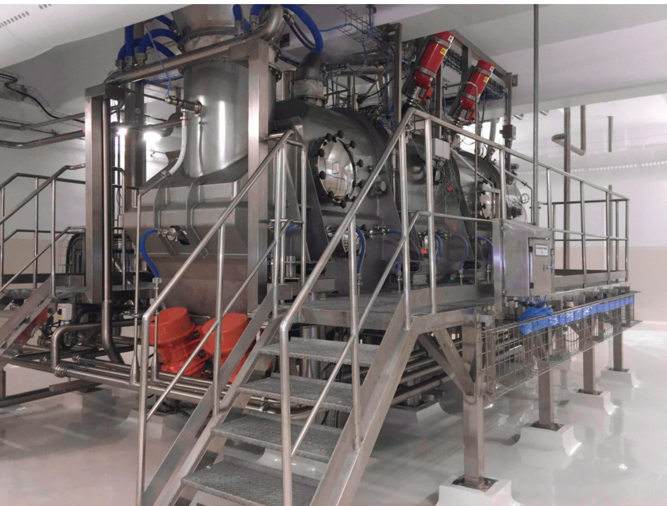
Vibrating fluid bed cooler-conditioner.
