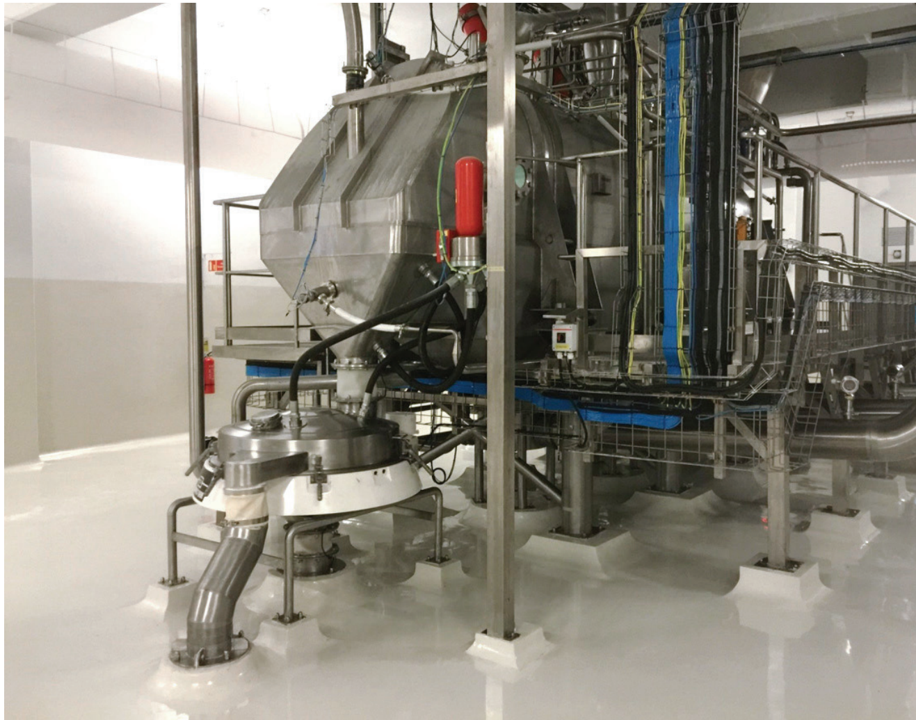
Fluid bed discharge with sifter.
