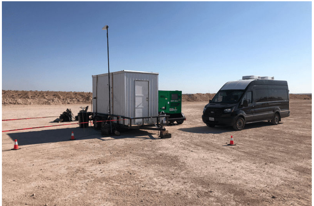
Fiber optic data acquisition units on a remote well pad location. Photo courtesy of Neubrex Ltd.
