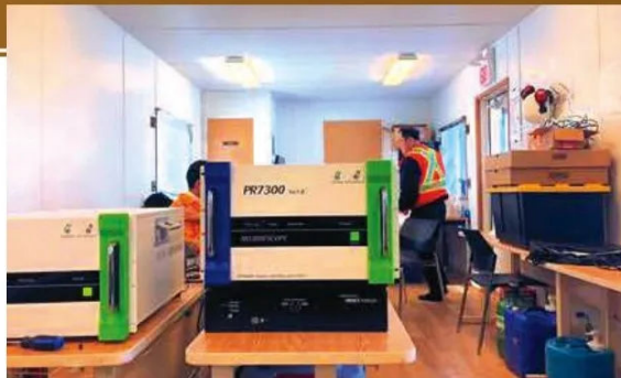
Neubrescope positioned on a negative-stiffness vibration isolator. Courtesy Neubrex Energy Services
