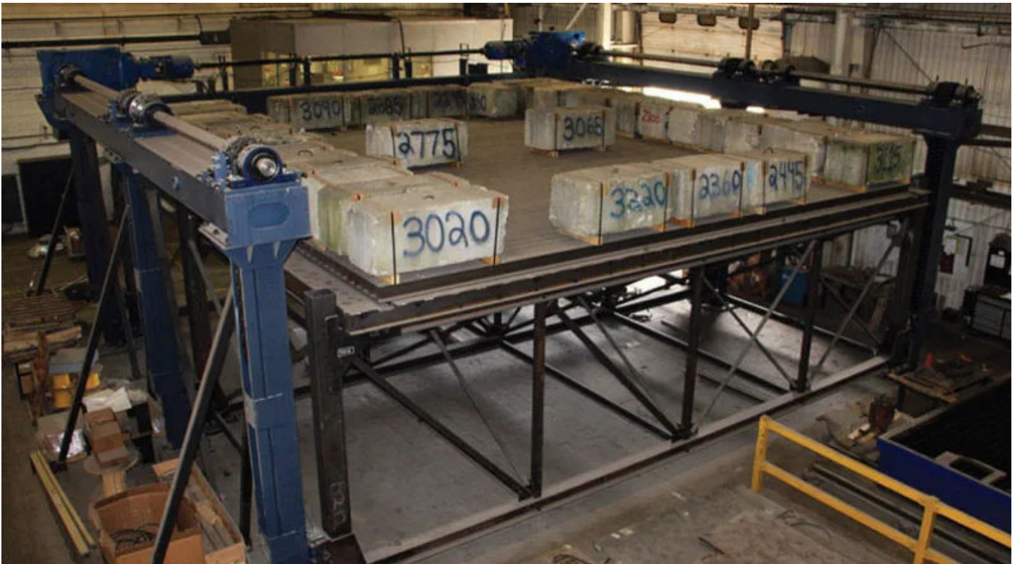
Testing the 35 x 35 x 11' lift carriage assembly at Pflow facilities.
