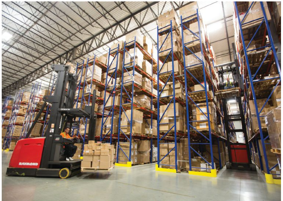
New merchandise is processed in the receiving area and then delivered to a staging area for putaway in the very narrow aisle storage area.
