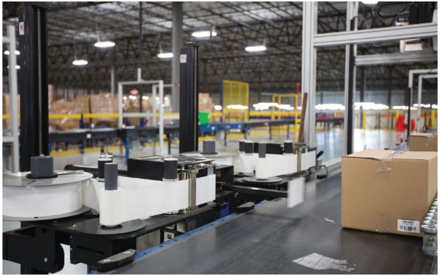
Automated print-and-apply technology has replaced the manual labeling processes that were used in the old facilities.
