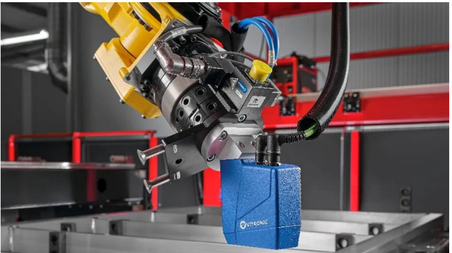
Inspecting weld seams on an automotive battery frame using automated vision inspection. VITRONIC Machine Vision
