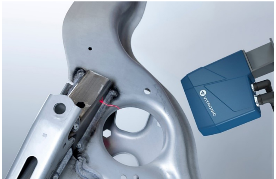
© VITRONIC Machine Vision | https://www.vitronic.com/ VITRONIC VIRO WSI inspects weld seams on an axle carrier for a Tier-1 supplier.
