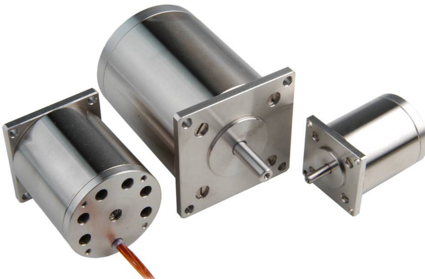
Figure 3: Typical motors for UHV applications: outgassing holes, polyimide-shielded braids, and clean stainless steel surface. Courtesy: PI
