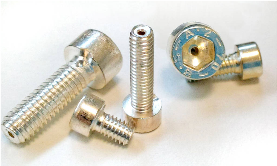
Figure 5: Example for Design-for-Vacuum: Drilled silver-plated screws for venting of trapped volumes in vacuum. Courtesy: PI
