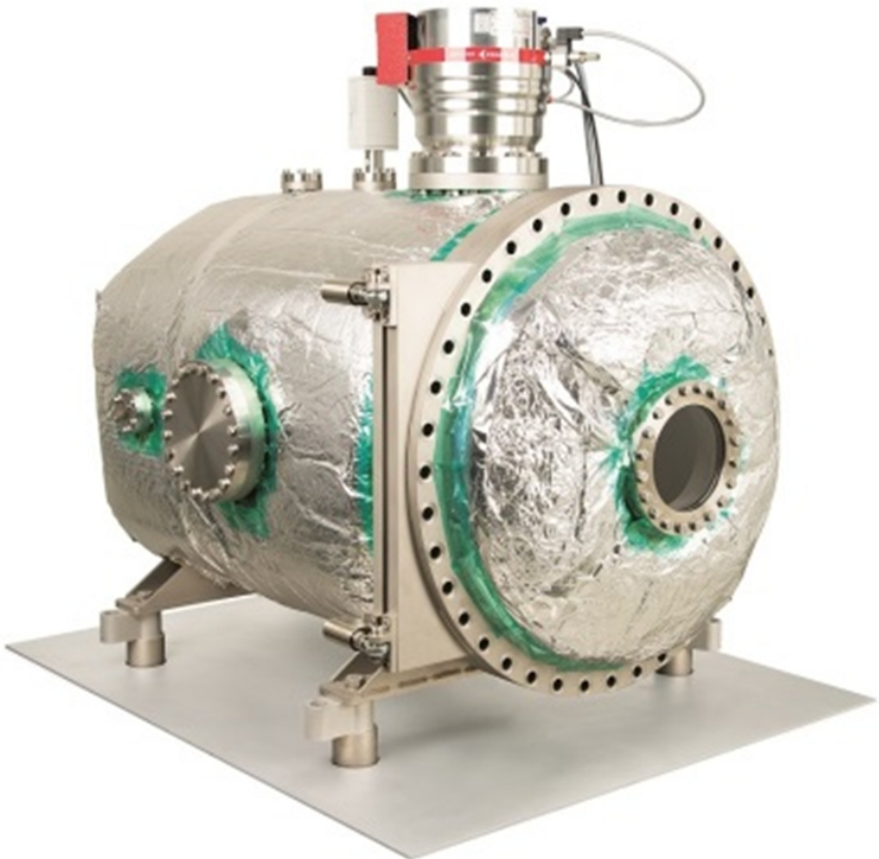
Figure 6: Large vacuum chamber test facility at PI. Courtesy: PI
