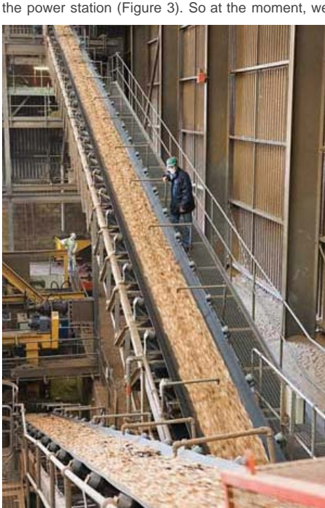
3. Wood chips being conveyed from storage to the plant's two circulating fluidized bed
