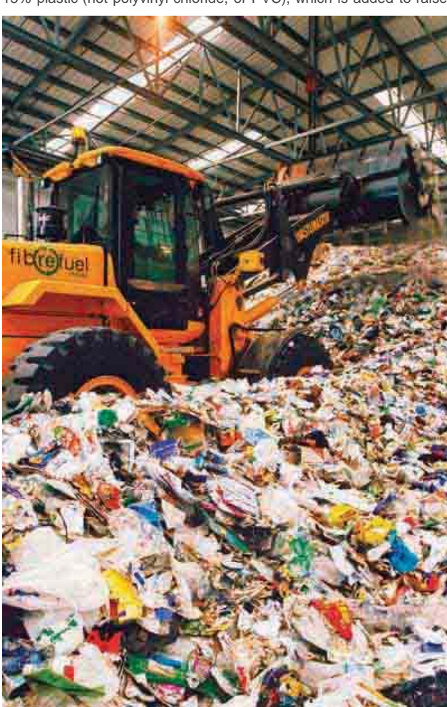
5. Nonrecyclable waste ready to be converted to fuel by an on-site processing plant operated by a dedicated utility subsidiary. Courtesy: Slough Heat & Power
