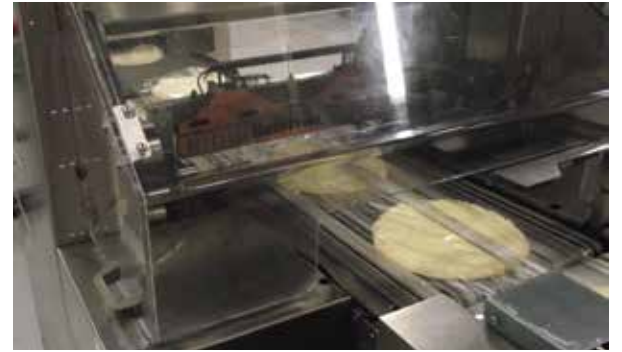
Bagged frozen pizzas entering the plant's newly-installed Texwrap shrinkwrapper.
