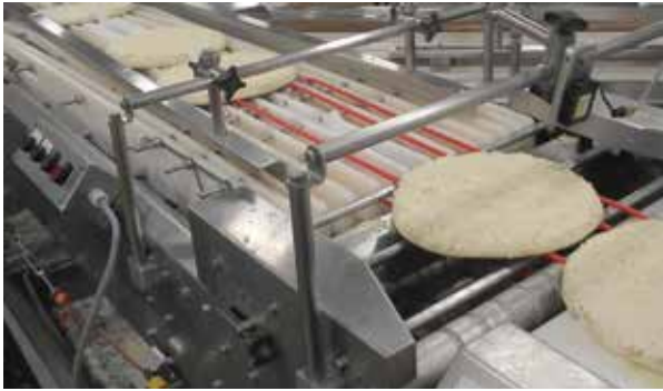
Frozen pizzas being spaced out for loading inside the plastic shrinkwrap bags.
