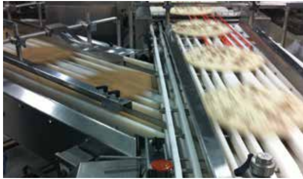
Pizzas and supporting cardboard disks being matched up before entering the shrinkwrapper.
