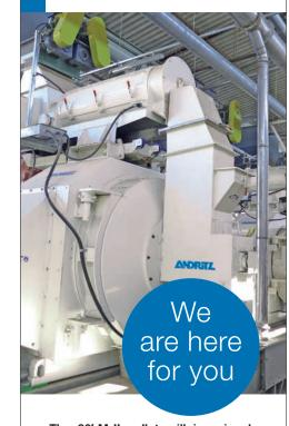
The 26LM-II pellet mill is uniquely designed to provide higher performance at the industry's lowest operating costs, and it is successful in the very demanding task of pelleting biomass materials. The office and workshop in North America specializes in the production of high quality ANDRITZ machines and equipment for the feed industries. We are proud of our long history and strong commitment to serve our customers.
