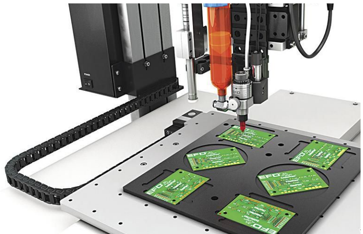
Because the needle must move up and down to contact the substrate, contact dispensing is slower than jet dispensing. Contact dispensing typically maxes out at approximately 300 deposits per minute. Photo courtesy Nordson EFD
