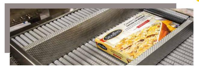
Because of the unique features of Slip-Torque rollers. the conveyor system is a safe environment for workers that work near and interact with the trays being carried on the conveyor system. The roller contact surface is designed to stop immediately if a hand is placed on it. thus maintaining a safer working environment.
