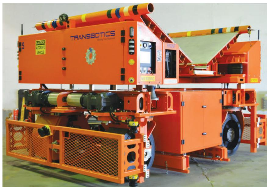
such as 60,000-pound aluminium coils, 120,000 pound steel ingots, or heavy loads with weights of over 200,000 pounds – have typically been designed so that the weight of the AGV is 40 to 60% of the expected load. An AGV engineered to carry a 60,000-pound aluminium coil, for example, would have a designed vehicle weight of between 25,000 to 35,000 pounds. This 40/60% ratio has been the conventional AGV design for decades.
